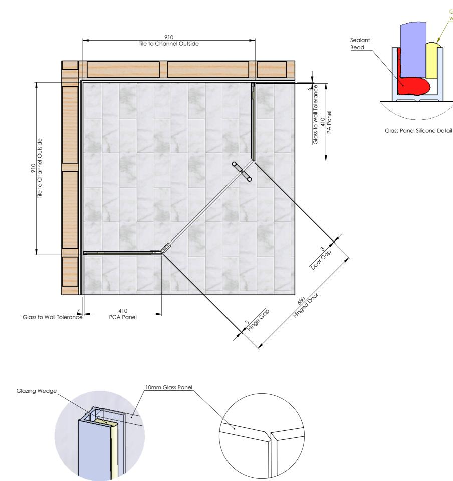
Glass To Wall Tolerance DETAIL A
