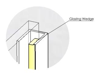
Glass To Wall Tolerance DETAIL B
