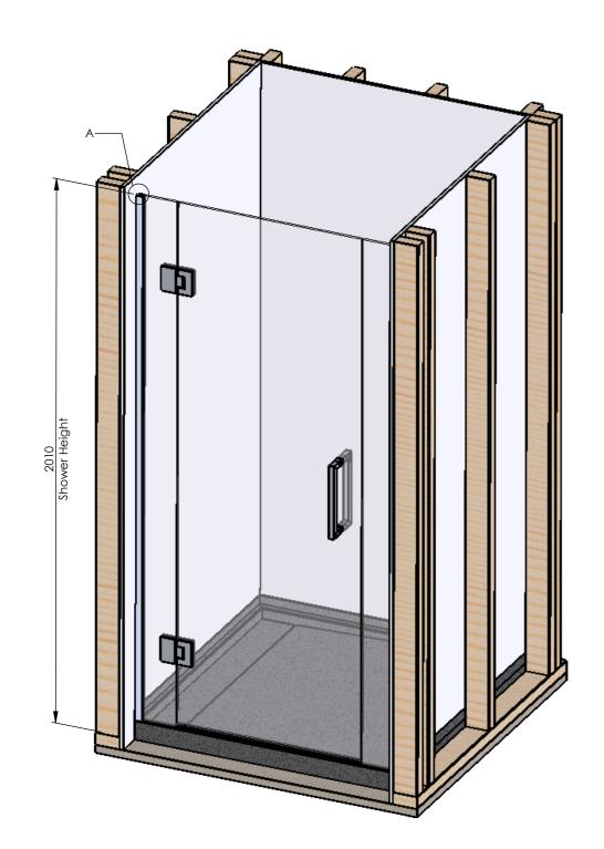
Framing/Base Outside 92 - Waste Centre 502 - Waste Centre 1004 Framing/Base Outside 9 Glass to Wall Tolerance 9 Glass to Wall Tolerance 3 - Door Gap 680 - Hinged Door
